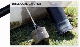
The drill core is held securely on the feed rod and can be easily removed.
